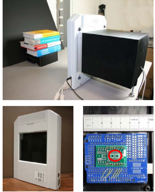
Figure 2. Prototype device. Top: lab setup. Bottom left: the LCD screen as the aperture assembly. Bottom right: the sensor board with two sensors, indicated by the red circle.
